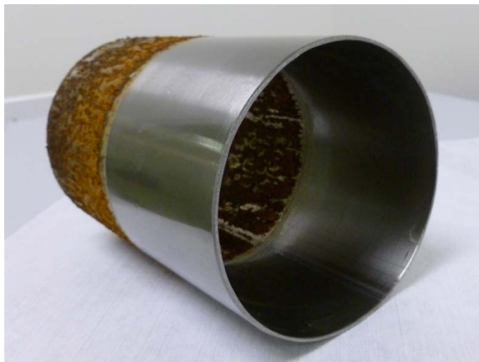
Fig. 1A photograph of a 10 cm steel pipe, half-coated with F coating internally and externally, and subjected to accelerated corrosion.
